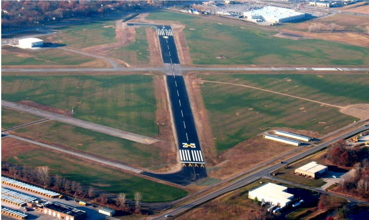
Figure 2-3. Markings for a Temporarily Closed Runway
